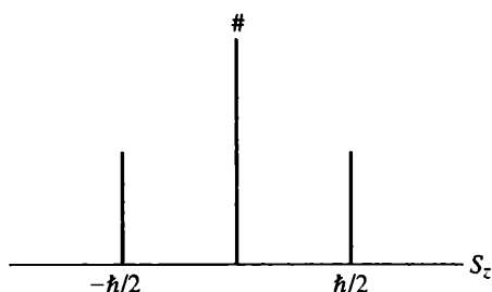
Figure 1.8 An idealized set of data resulting from measurements of S_z on a collection of particles with S_x = \hbar/2 .
